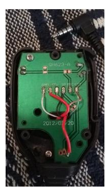
Other users report varying pinouts. The mic is much easier to open than the radio itself, and the pin configuration is often silk screened on the PCB. Use a multi-meter to trace the wires to the TRRS head to determine your pinout.
